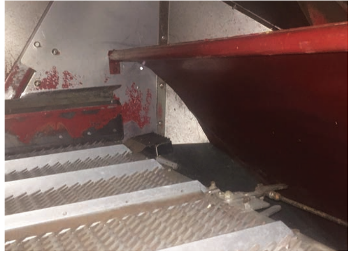
FIGURE 12 Separator baffle in a Case 2388 sitting approximately 300mm above the rear of the sieve.
