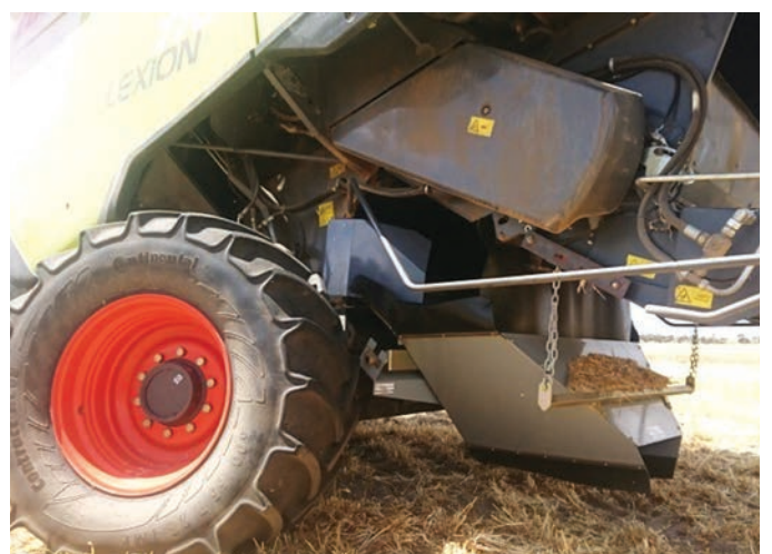
FIGURE 27 Claas Lexion chaff line chute – Westoz Boilermaking.
