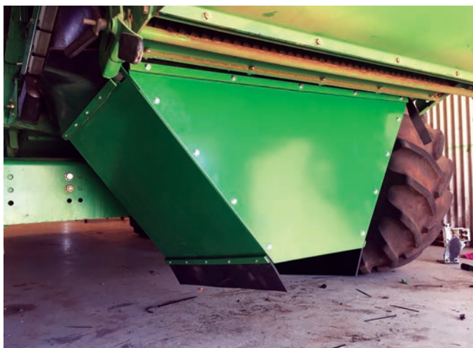
FIGURE 19 S-series John Deere chaff line chute – Westoz Boilermaking.
