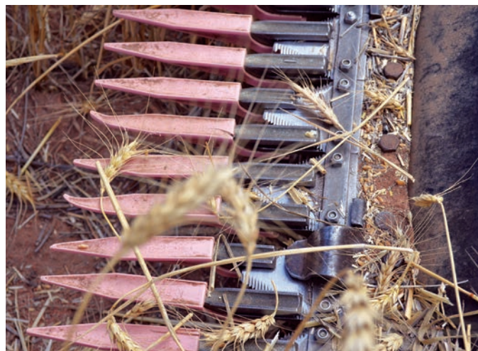
FIGURE 2 Primary sales knife extensions used to improve crop and weed seed capture.
