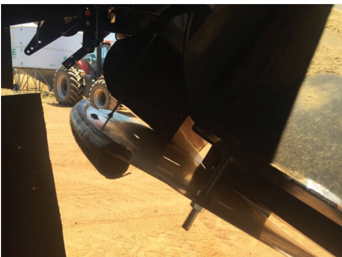
FIGURE 15 Another 'Rod and Andrew Messina' straw spreader cover fitted to a Case 8230 owned by Craig Simkin from Binu. The height of this baffle is adjustable with slotted holes, allowing for 100mm of height adjustment.
