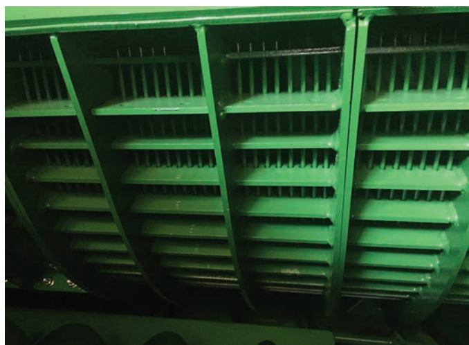
FIGURE 5 A standard John Deere 31 wire concave. Manufacturers recommend all three concave sections to be 31 wire for normal cereal harvesting.
