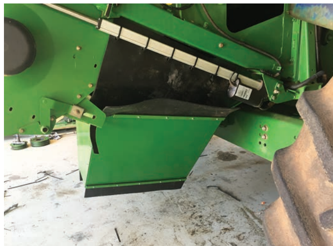
FIGURE 20 Side view of the S-series John Deere chute – Westoz Boilermaking. The chopper slides back on the rails. The chopper sensor is moved to allow the chopper to continue to operate when in this position. An overshoot beater is a good idea to help throw straw further back into the chopper.
