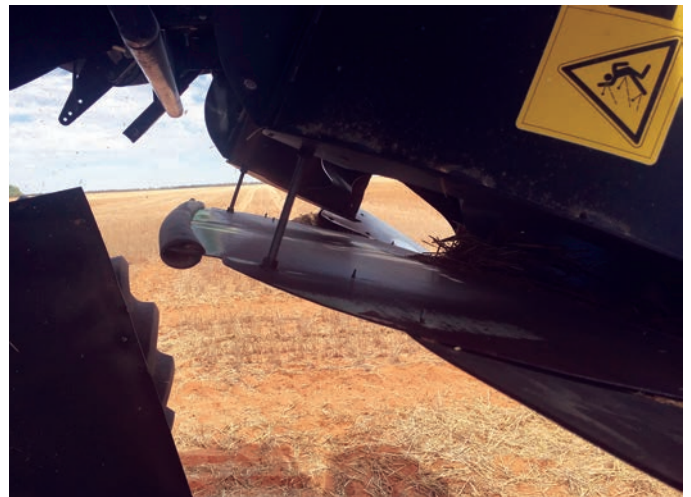
FIGURE 14 Straw spreader cover fitted to a Case 7230 owned by Craig Thompson, north-eastern wheatbelt of WA. Commonly known as the 'Rod and Andrew Messina' design, as this is what they used as a baffle with chaff carts fitted. This is designed to cover the front of the straw spreader so that the weed seed-bearing chaff is not sucked into the straw spreaders.
