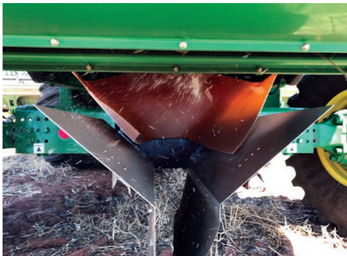
FIGURE 29 Rear view of Matt Johnson's chaff line chute, showing the shaking plastic IBC chute feeding into the fixed steel chute. Rubber sides on the bottom of the chute reduce crosswind effects.
