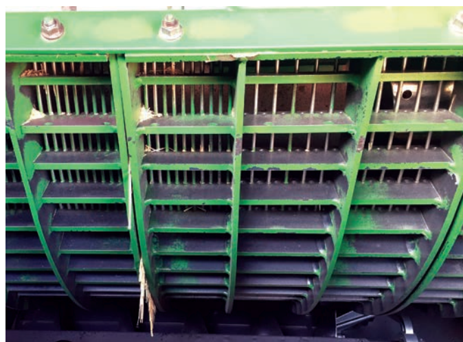
FIGURE 6 The first section of concave is a standard 31 wire for aggressive threshing, leading into the next section where every second wire is removed to allow grain and weed seeds to exit the rotor.
