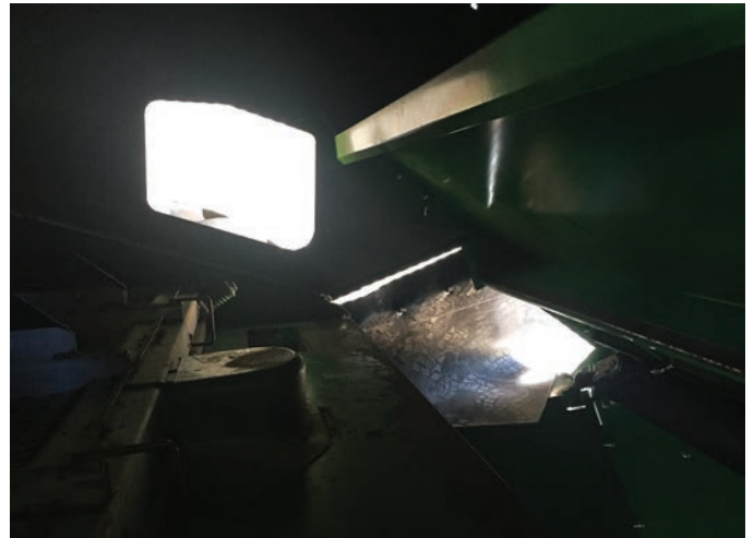
FIGURE 10 Separator baffle inside a John Deere harvester leading into a chaff line chute made by Westoz Boilermaking.
