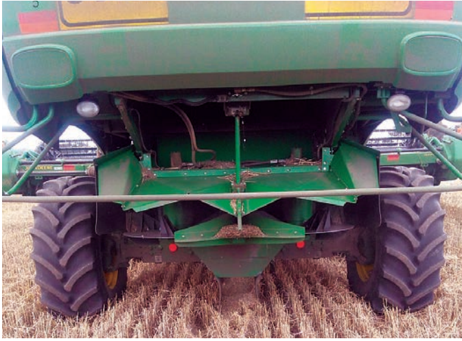
FIGURE 33 The Kohlhagens' chaff line chute in action on a John Deere S670. The straw spreaders are in the normal 'down' position.
