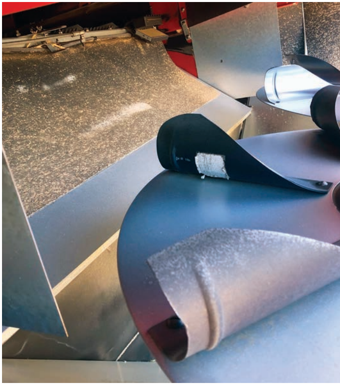
FIGURE 39 Residue delivery onto the spinners.
