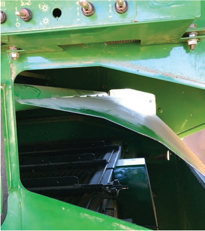
FIGURE 32 The Kohlhagens' chaff line chute on a John Deere S670. This photo shows how the tray behind the sieve was removed to create some room between the sieve and the straw spreaders. The baffle is curved with a rounded leading edge, and a new cover has been made for the sieve controlling mechanism.
