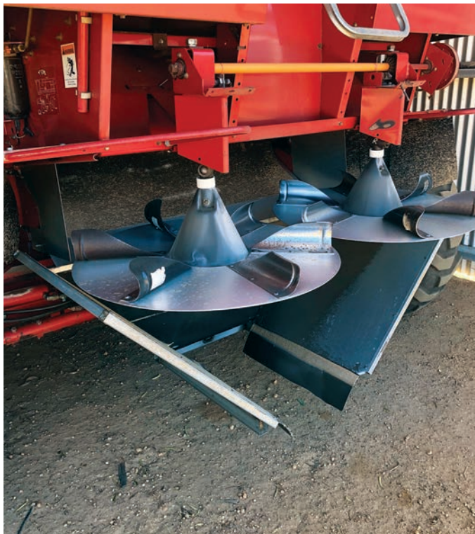
FIGURE 36 Chaff line set-up on Rowan Astbury's Case 2388 with straw spreaders moved back 150mm and up 100mm.
