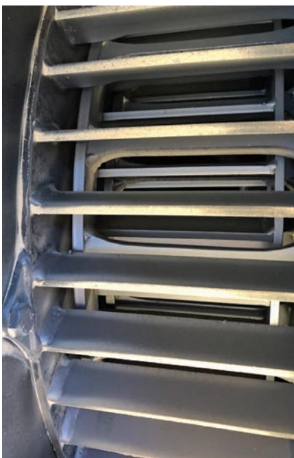
Mill wear after 1000ha canola at 1.2t/ha, 1000ha of barley at 3.5t/ha, 250ha wheat at 3t/ha.
