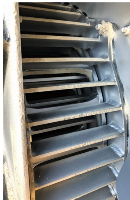
Mill wear on a New Holland 10.90 after 900ha of canola at 1.3t/ha, 1200ha of barley averaging 3t/ha.
