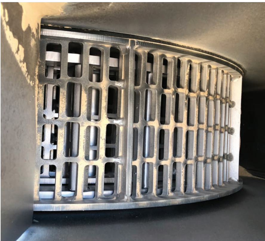
Mill wear on a John Deere S680 after 200ha of beans at 2t/ha, 400ha of canola at 1.5t/ha, 230ha of irrigated canola at 4t/ha, 550ha of barley at 5.5t/ha and 60 ha of wheat at 6t/ha.
