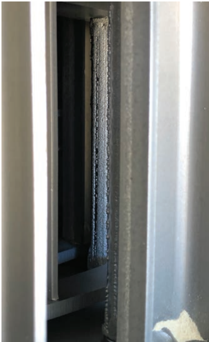
Mill wear on a John Deere S680 after 100ha lupins at 1.8t/ha, 600ha canola at 1.2t/ha, 700ha frost affected barley at 2t/ha (3.5t/ha stubble), 1100ha frost affected wheat at 2t/ha (3t/ha stubble).
