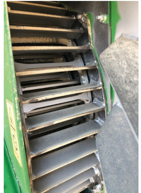
Mill wear on a John Deere S680 after harvesting 650t of barley, 2580t of wheat, 225t of canola and 100t of oats.
