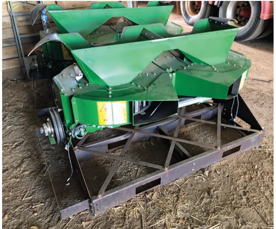
A folded steel frame that bolts to the SCU for forklifting off is a neat arrangement making mounting and removal safer and more simple.
