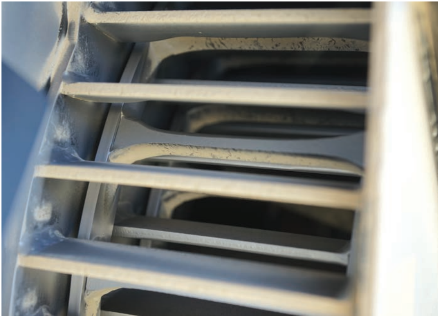
Mill wear on a Case IH 9120 after 800ha barley averaging 1.4 t/ha, 1700ha of frost affected wheat averaging 1.3 t/ha.
