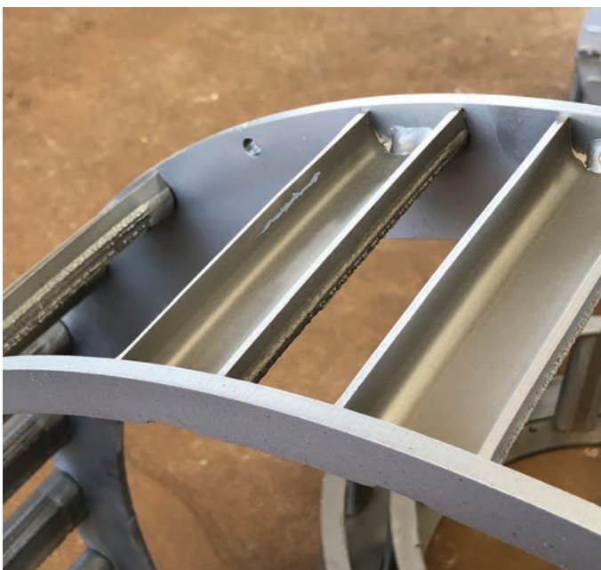
Mill wear on a John Deere S790 after 400 hours of operation at Wongan Hills, WA after 3700ha of wheat, barley, canola and lupins.
