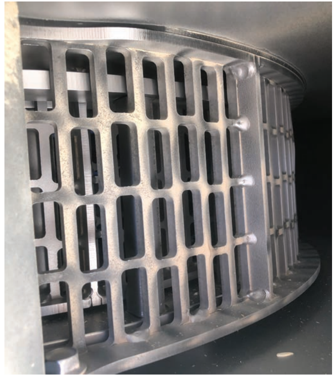
Mill wear on a Case IH AFS 7240 after 1000ha of frost affected wheat yielding 1.7t/ha, 500ha of canola averaging 1.2t/ha.
