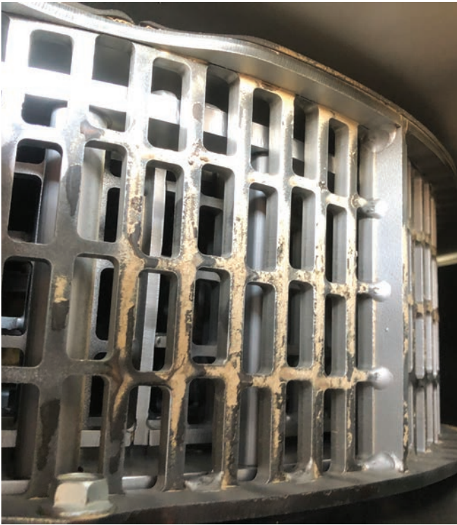
Mill wear on a John Deere 9770 after harvesting 650t of barley, 2580t of wheat, 225t of canola and 100t of oats.
