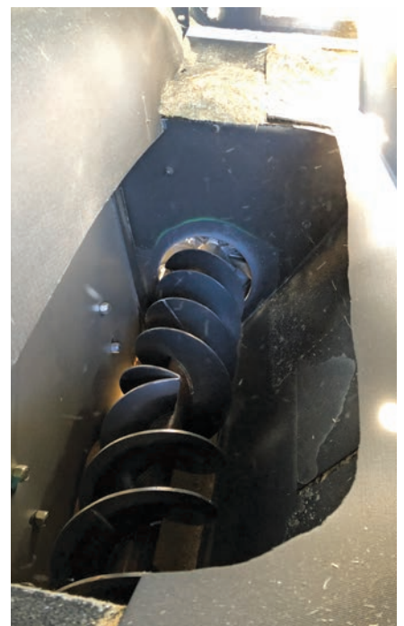
Lateral auger feeding each of the mills.
