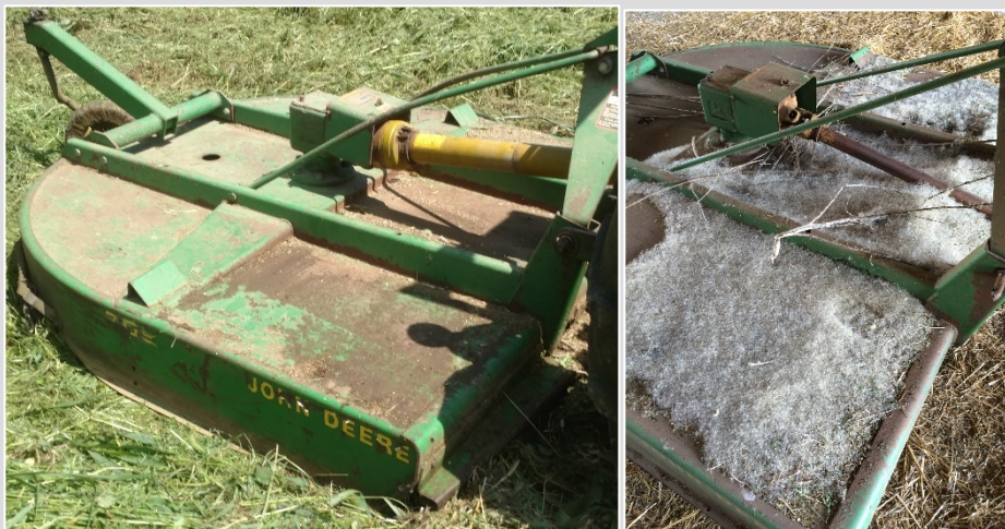
Photo 6.1: Cleaned brush mower (left) versus a brush mower covered in dandelion seed (right) (Photo credit: M. Flessner).
