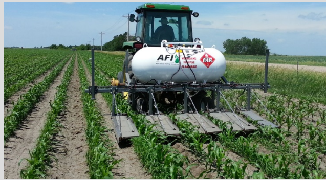
Photo 11.2. Flame weeder with torches under hoods to improve safety of the crop and prevent heat from dissipating too quickly (Photo credit: Agricultural Flaming Innovations).
