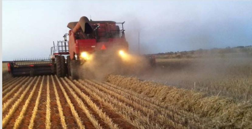
Photo 15.1. Chaff being formed into windrows during harvest in preparation for narrow windrow burning in a western Australia wheat field (Photo credit: R. Messina and A. Messina, ABC News Australia).
