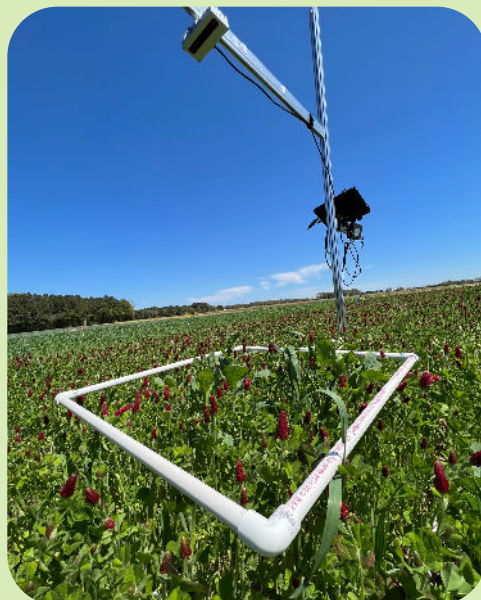
Figure 17. The OAK-D multisensor camera, being tested by GROW, combines an RGB camera for object detection and identification, with a stereo camera that provides depth mapping capability. Combined with computer vision models trained on large image datasets for individual crop and weed species, the OAK-D allows for the estimation of plant density and biomass at the species level. (Photo credit: Claudio Rubione, GROW.)
