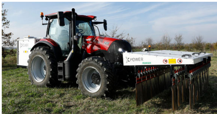
Figure 3. A Zasso XPower continuous-contact electrical weeder. (Photo credit: Case IH)
