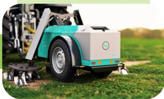
Figure 9: RootWave electrical weeder for use in orchards and vineyards. (Source: RootWave 2024)
