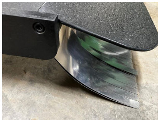
Figure 4. Close-up image showing the electrodes of a Zasso continuous contact electrical weeder. (Photo credit: Lynn Sosnoskie, Cornell University)
