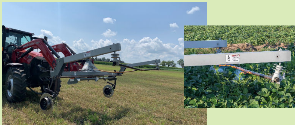
Figure 2. (Left) Full view of a spark-discharge unit in the field. (Right) A spark-discharge electrical weed control tool at work in soybeans to target waterhemp escapes that have grown above the crop canopy. (Photo credit: Ryan Hamberg, Texas A&M; Kevin Bradley, University of Missouri)
