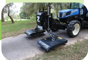
Figure 8: Zasso XPower XPS (top) and E-Coffee (bottom) electrical weeders. (Source: TJ Lange/Burrows Tractor, 2024; Zasso, 2024)
