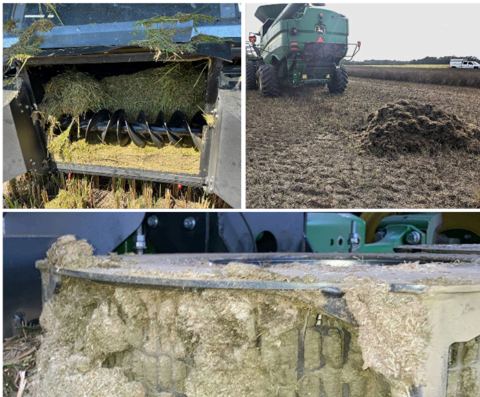
Figure 4: Clogged plant material in seed impact mills. Clockwise from top left: purple ammannia in rice harvest blocking an iHSD, a clog ejected from a Redekop SCU during soybean harvest, and a Seed Terminator clogged with wet plant material. (Photo credits: Sarah Chu, Texas A&M, Claudio Rubione, GROW, and Josh Lade, JET Farms Ltd.)
